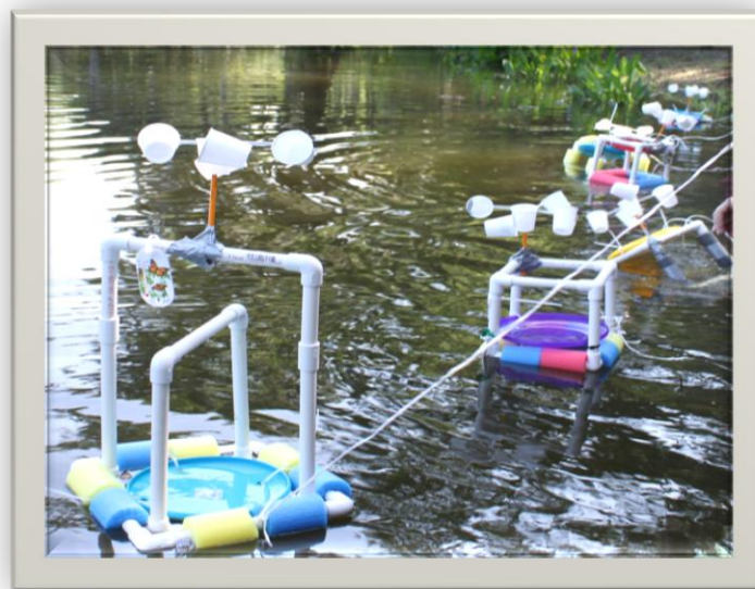
In the figure above, eBOBs outfitted with student made anemometers and thermometers are tethered and deployed in a Charleston pond.
