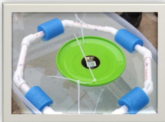
An octagonal option for eBOB in a Bag that is outfitted with the flying disk platform and ready for the eBOB Payload Challenge .
