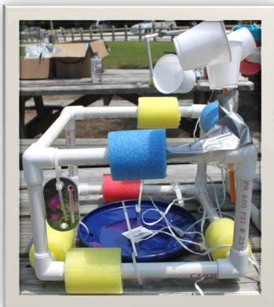
eBOB outfitted with student-made anemometer and air thermometer.
