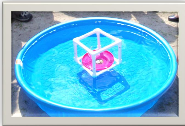
eBOB stability and buoyancy being tested during the eBOB construction phase.
