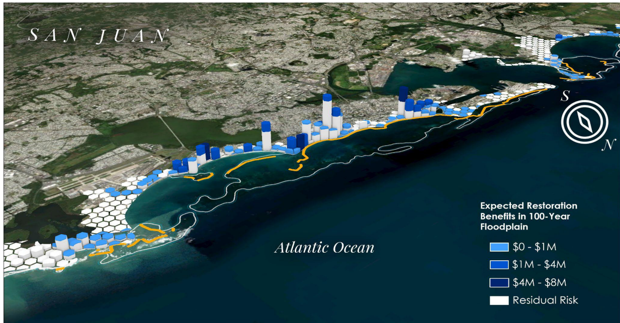
Figure 17. Risk reduction benefits of reef restoration around San Juan, Puerto Rico. The full height of the bars indicates current expected flood risk in the 100-year floodplain. The blue bar tops indicate the risk that could be reduced with reef restoration; their height and color represent the expected benefit from restoration per 50,000 m 2 (hexagon max width = 277 m). Residual risk remains even after reef restoration. The orange line offshore indicates the location of potential reef restoration. The offshore polygon outlined in white represents the extent of current reef habitats. Modified from Storlazzi et al. (2021).
